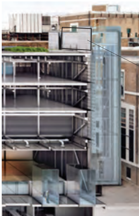
A rendered view and perspective section fragment of the circulation tower, which the curtain wall surrounds.
