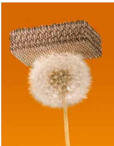
The new nickel-phosphorus lattice is as light as a feather, © HRL Laboratories, LLC/Photo by Dan Little
