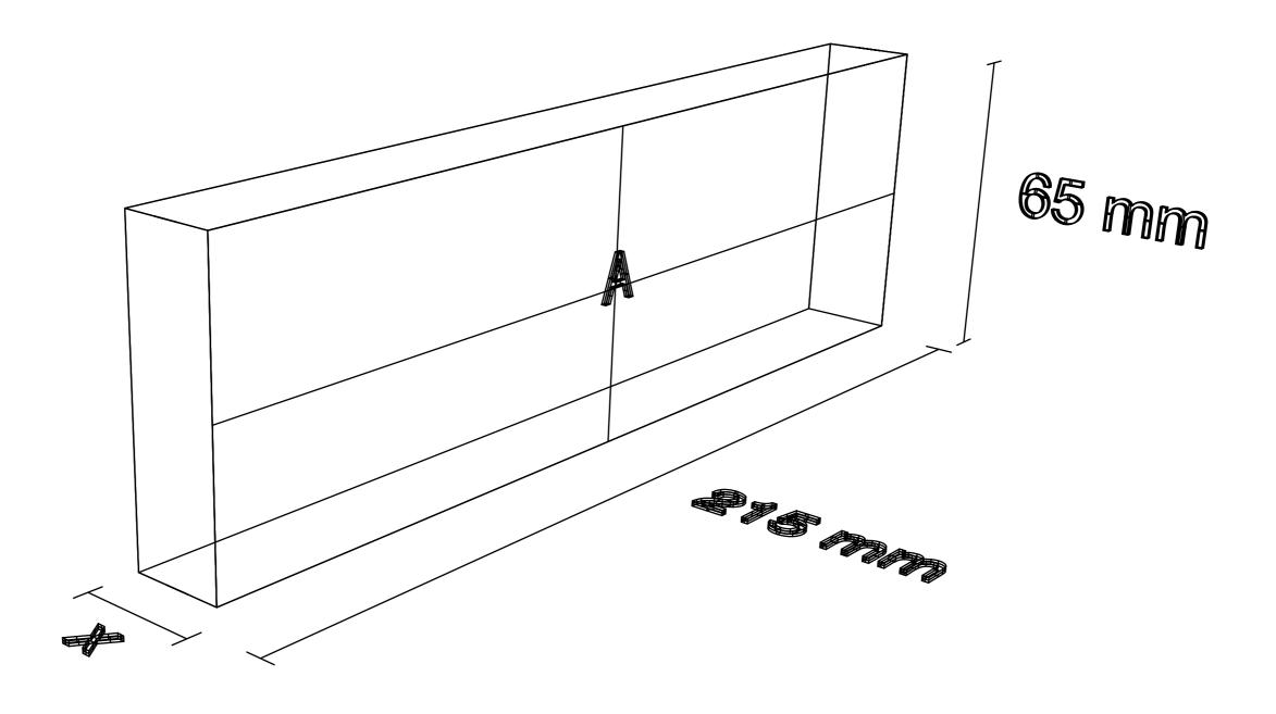
Following from that, the 'feather brick' must be only 19.33mm thick (x=19.33) in order to be equally thermally efficient as a standard brick used in typical London facades.
