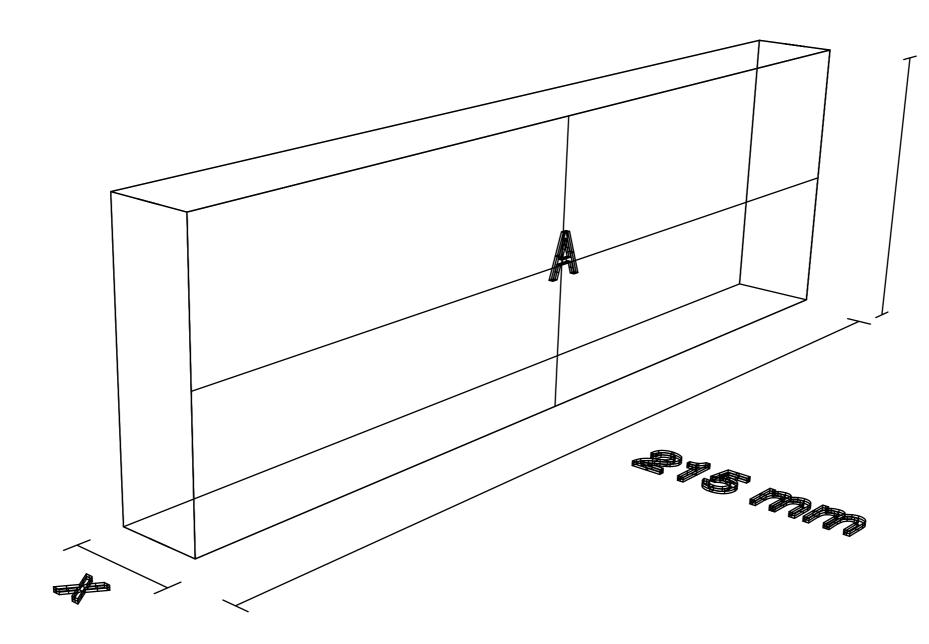
Following from that, the 'feather brick' must be only 19.33mm thick (x=19.33) in order to be equally thermally efficient as a standard brick used in typical London facades.
