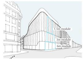
Six meter modules of flat and curved glass elements define the retail facade to ground and first floor. The upper floors are articulated by three meter modules with the variation in width taken up by flat glass panels, allowing the bespoke curved elements to remain the same throughout. The two top floors are composed of curved panels in 1.5m bays with one curved panel directly adjacent to another.
