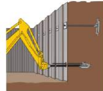
Sheet piles installation
