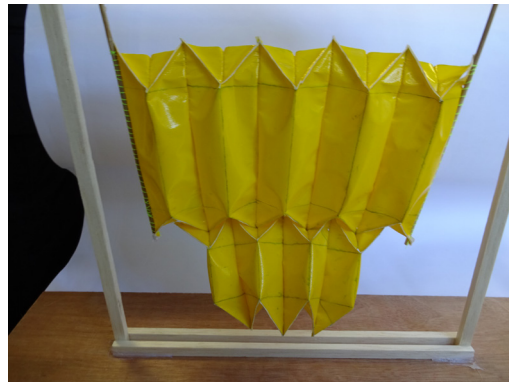
When stretched, the lower part tilts to create a rain cover
