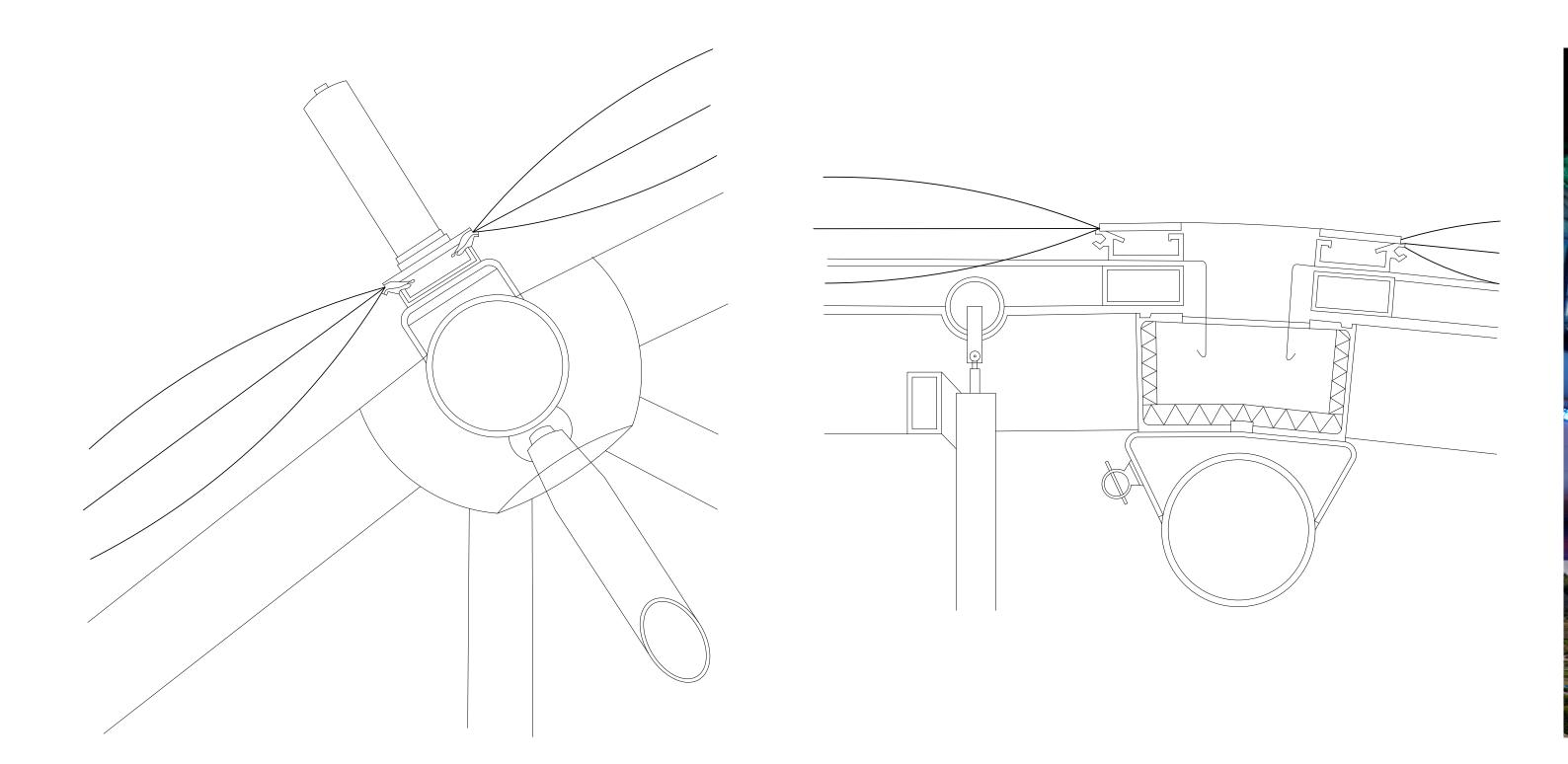
Each dome has what's known as a hex-tri-hex space frame with two layers. The outer layer is made of hexagons (the largest is 11 metres across), plus the odd pentagon. The inner layer comprises hexagons and triangles bolted together. The steel-work weighs only slightly more than the air contained by the Biomes. The structures are more likely to blow away than down, so are tied into the foundations with ground anchors, a bit like tent pegs.
