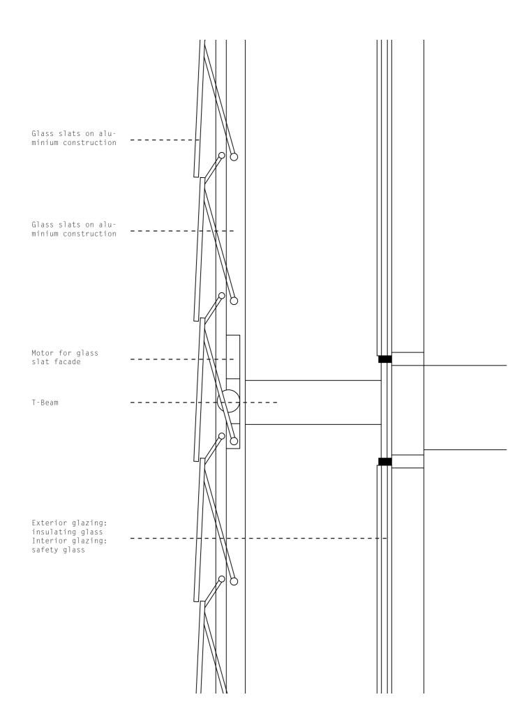
The facade is made of double-layer glass: The inner glass is full length from floor to ceiling. The outer layer is made of glass panels that open and close to manage ventilation and insulate heat in the winter and let out heat in the summer.
