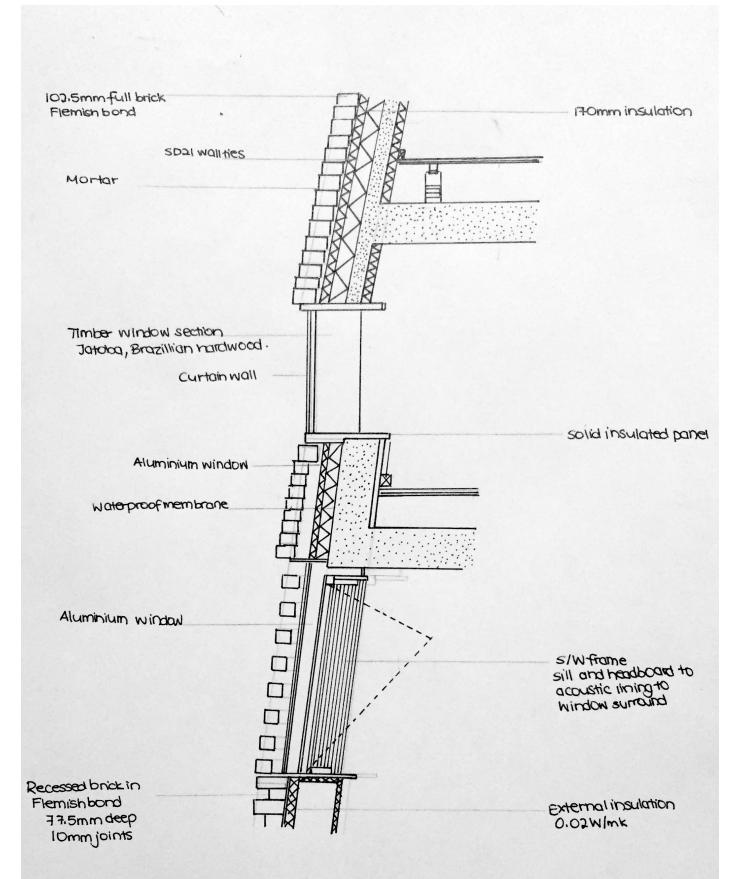
The faceted facade consists of solid brickwork, open latticed brickwork and glazed timber screens. The open lattice is a punctured Flemish bond with headers removed for light and air ventilation, also providing solar shading. Solid brickwork is in place where day light and ventilation are not required. This clads the concrete structure and insulated cavity.
