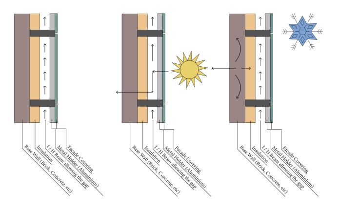
Ventilated type facade and wall coverings were developed to protect buildings against the combined action of different types of weather. This is done by counterbalancing the effects of water beating on walls and keeping the building dry, with high level aesthetic characteristics. Moreover the facade has undisputed advantages of heat insulation and soundproofing.
