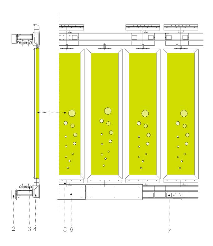
1.Solar leaf external louvre 2.Brackets with thermal breaks for the transfer of loads to the primarysubstructure 3.Pipework for the medium to enter and leave 4.Sub-frame, rolled steel U-section 5.Pivot fixing allowing rotation 6.Metal cladding 7.Supply of pressurised air, controlled by magnetic valves
