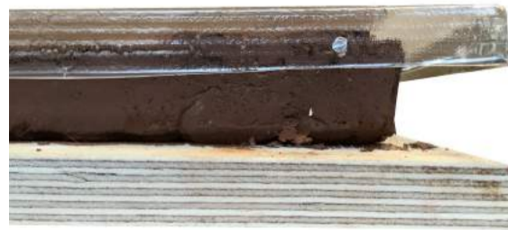
Nail connection between the thermoplastic and the brick
